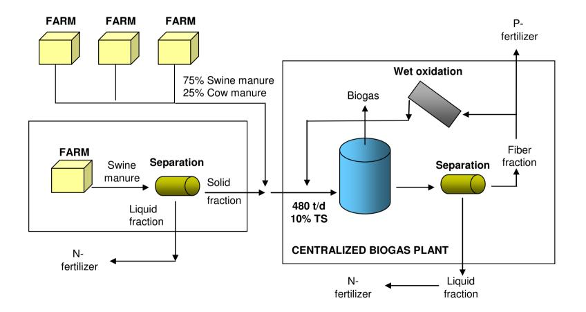
Scenario 2a, On farm separation, dry matter content 10%, pressure boiling of post separated fibre fraction
